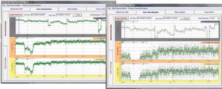
**FIG. 4** Autonomous cleansing and summarization of high-frequency data and online, adaptive modeling of high-frequency data streams. Data is from an oil-producing carbonate reservoir in the Middle East.
