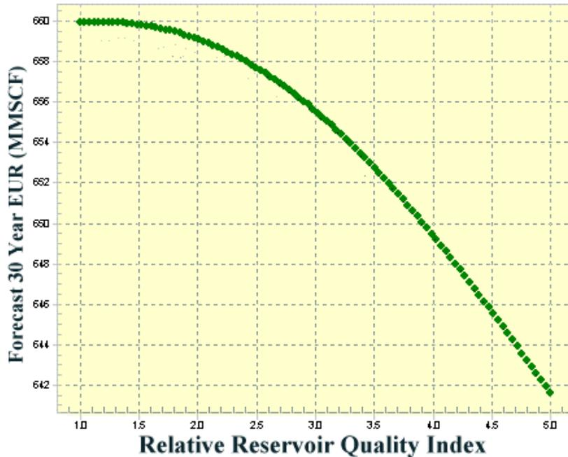
**Figure 4.** Sensitivity of Forecasted 30 Year EUR to Relative Reservoir Quality Index (RRQI) for a well in the database. RRQI is lower for the better parts of the reservoir.
