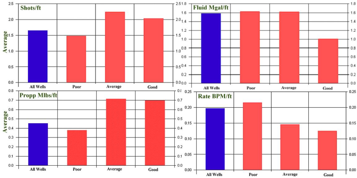
**Figure 12.** Distribution of the average value of completion parameters in wells of different quality.
