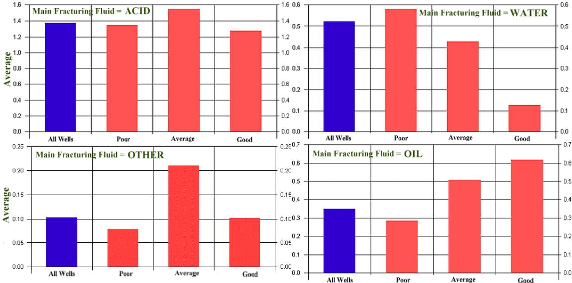
**Figure 11.** Distribution of the average value of Main Fracturing Fluids in wells of different quality.
