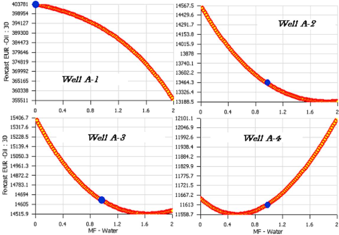
**Figure 18.** Sensitivity analysis for water as the main fracturing fluid for four wells in the database.
