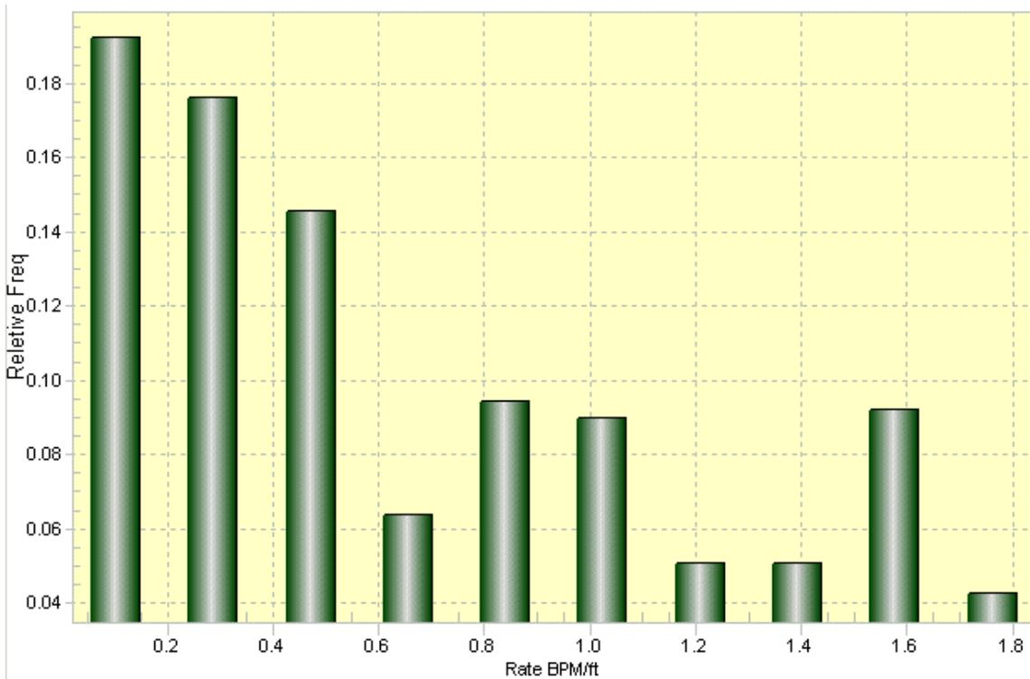
**Figure 5.** Frequency distribution of injection rates in BPM/ft for the top solutions during the optimization process.
